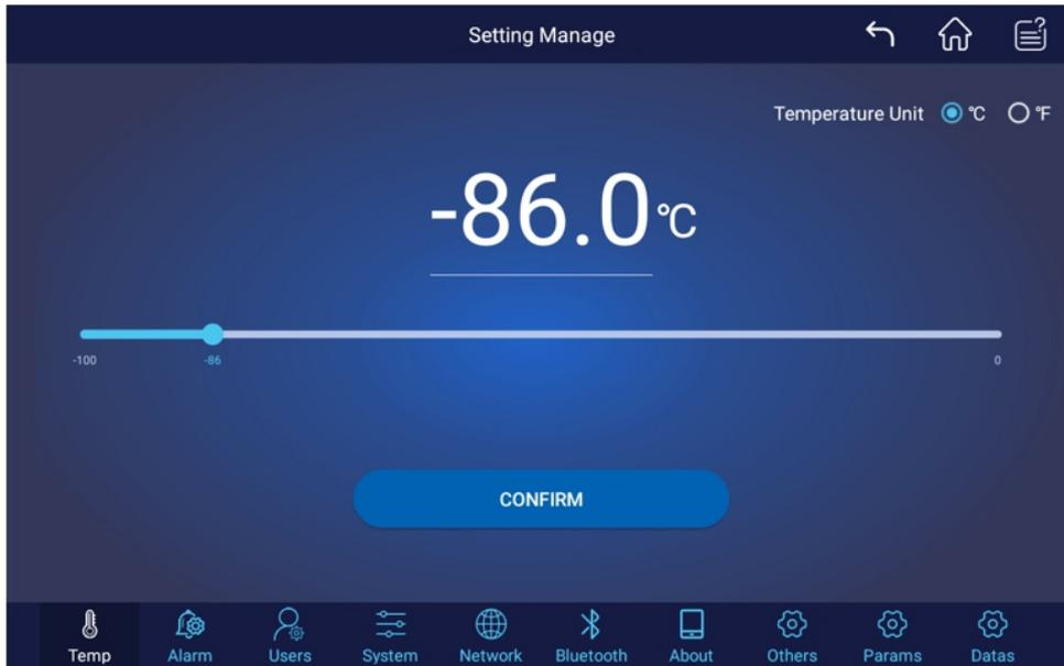
a. Temperature setting. You can slide on the slider or click the temperature value to modify the set temperature, and click the °C (Celsius temperature scale) or °F (Fahrenheit temperature scale) to switch the temperature scale;
