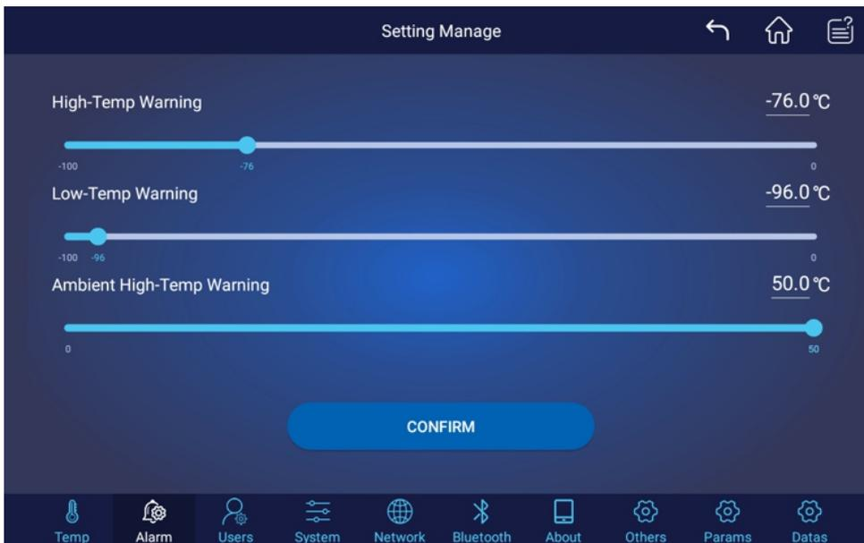
b. Alarm setting. You can slide on the slider or click the value to set the high-temperature alarm value, the low-temperature alarm value, the high ambient temperature alarm value;
